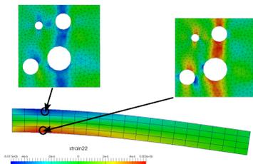
Figure 1: Computational homogenisation of the micro-structure to resolve a cantilever beam
